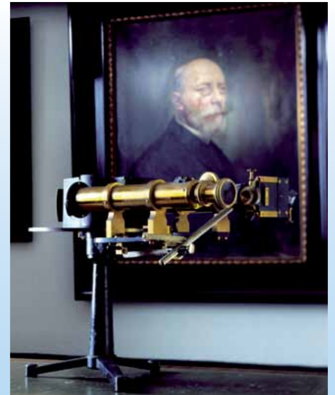
Astronomical direct vision spectroscope in front of the portrait of professor Hugo Krüss.
